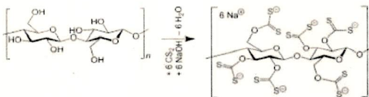
Figure 2-1. Treatment of Cellulose with Alkali and Carbon Disulfide to Yield ORC
